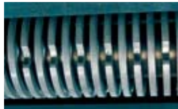
The special groove form of the cutting and perforation rollers ensures particularly effective padding
